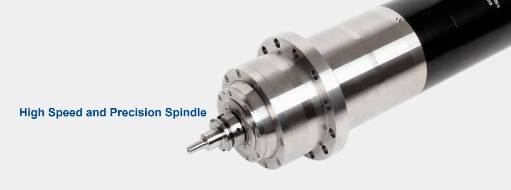
High speed and precision spindle is the key part of Jingdiao machining centers that ensures process precise and efficient. High speed and precision spindle has many advantages such as compact structure, large speed range, high rotation accuracy, light weight, low inertia, slight vibration, and low noise etc.. The latest spindle has composite machining capabilities of milling, holes drilling, thread tapping, turning, grinding, polishing and scraping etc..
